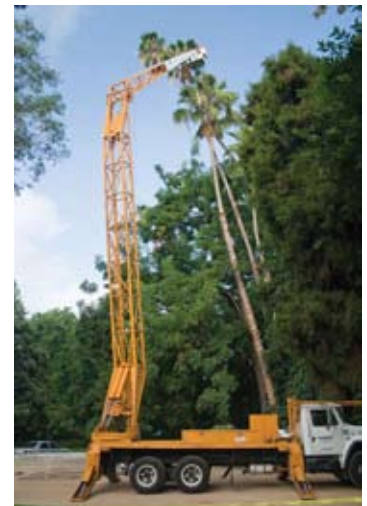
Figure 26. Where appropriate, the use of mechanical lifts and tower bucket trucks to prune even the tallest palms, such as these Washingtonia robusta , is safe, reliable, and non-damaging to the palm.
